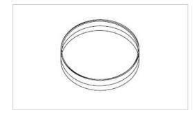
Dish height 13.5 mm, dish diameter 56 mm. Lid with triple venting protrusions.
