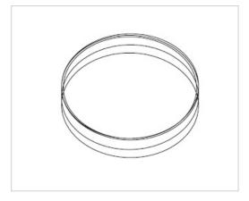
Dish height 14.5 mm, dish diameter 86.5 mm, wall thickness 1 – 1,2 mm. Lid with triple venting protrusions.
